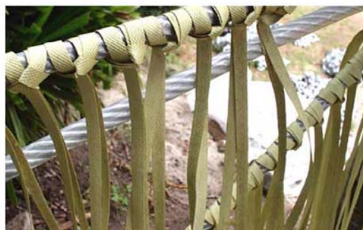
h) PVC-coated steel wire and 'aggregator' tape.
