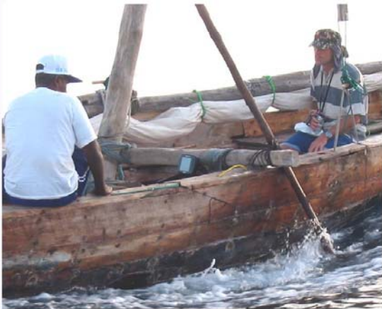
f) Echo-sounder mounting and screen.
