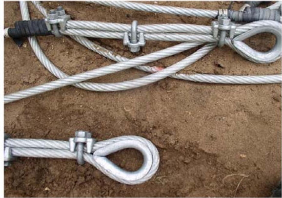
b) Cable clamps and thimbles on 16mm wire.
