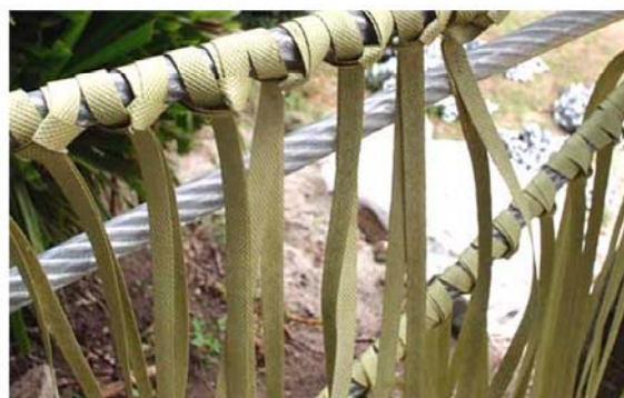
h) PVC-coated steel wire and 'aggregator' tape.
